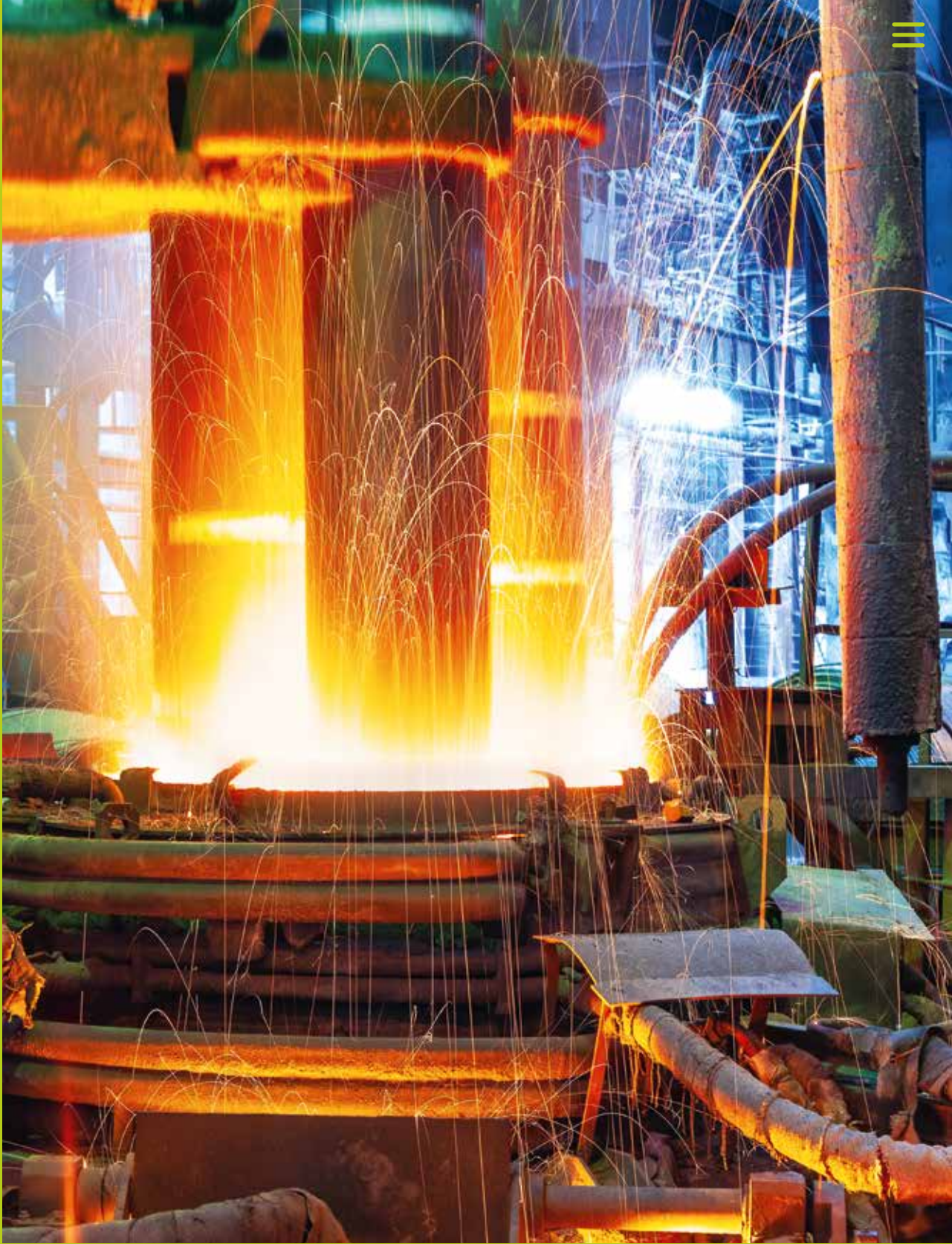
An electric arc furnace can be powered by green electricity.
